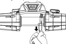
Once the rope has been pulled through, cut and discard the zip tie while being careful not to harm the rope.
