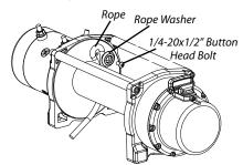
AWARNING Always wind the winch rope on bottom (mount side) of drum.
