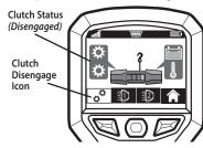
If clutch does not disengage when requested, a warning error will display within the clutch status icon. See Trouble Shooting section in this manual for possible solutions.
