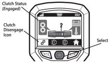
Once the clutch is successfully disengaged, the gears in both the clutch status and clutch disengage icon will change from "engaged" (2) status to "disengaged" (2) status.
