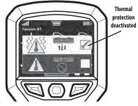
To activate the thermal protection setting, use the left or right button to highlight the thermal protection shut-off option. A check mark will appear in the box. Press select to confirm selection.
