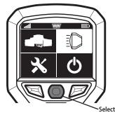
Auxiliaries can be switched on and off together using the Dual Auxiliary Icon or individually by using the Auxiliary 1 and Auxiliary 2 Icon and then pressing Select.
