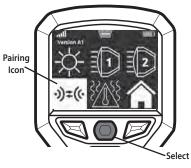
2. Press and hold select and the right button simultaneously for 3 seconds to bring up the pairing confirmation menu.
