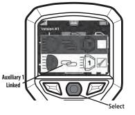
Note: Images show linking Auxiliary 1. Same process will be used for Auxiliary 2 linking.
