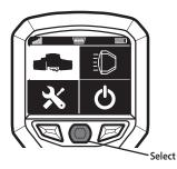
Following the Winch Activation Menu prompt, press and hold the Left and Right buttons simultaneously for 3 seconds to activate the Winch Operation menu.
