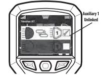
3. Using your left or right button to highlight the "linked" icon. A check mark will appear in the box. Press select to confirm selection.
