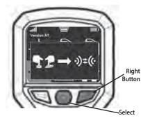
To continue pairing, select the green check mark icon by navigating with the left or right buttons and press Select.
