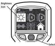
2. Use the Left and Right buttons to adjust slider to the desired brightness. Once the brightness is at the desired level, press Select to close the brightness adjust panel.
