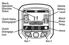
NOTE: The Winch Operation Menu is accessible from any menu by pressing and holding the left and right buttons simultaneously for three seconds.
