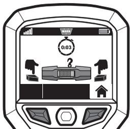
4. Disengage Clutch.
