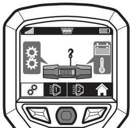
**NOTE:** The clutch will not disengage if the winch rope is under tension.
