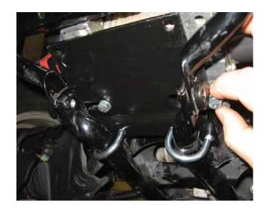
8. Push up on winch bracket to gain clearance for the second bolt to slide into the slot. Slide the winch toward center while aligning the second bolt with the slot.
