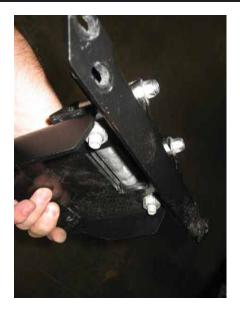
10. Install fairlead bracket UNDER winch mount plate.
