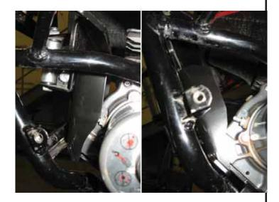
11. Align the upper winch holes with the upper holes in the winch mount bracket and fairlead bracket. In the motor side of winch, install ONE 8mm x 25mm long bolt and lock washer from Warn winch kit— do not tighten. For the other upper mounting hole, install an 8mm x 20mm long bolt and lock washer from Warn winch kit— do not tighten. Tighten lower bolts only to recommended torque specification on page 3. Push up on winch mount bracket if necessary to gain clearance for tightening.
