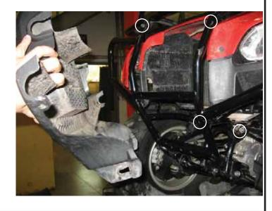
4. Install winch bracket using 8mm U-bolts and lock nuts. Tighten evenly and torque to specification shown on page 3.
