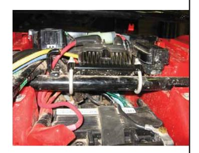
17. The suggested routing for the blue and yellow winch power cables is shown below. This routing requires removing the plastic from the right hand side and routing wires along the same path with the factory vehicle wires. Use cable ties and tape to secure power cables along routing.
