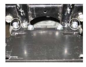
6. Partially install winch over mount bracket with the motor end first. Install ONE 8mm x 20mm long bolt and lock washer from Warn winch kit in lower hole – do not tighten. Leave bolt and washer loose enough to allow them to slide under winch bracket. Push up on winch bracket to gain clearance for the bolt to slide into the slot.
