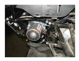
18. The suggested keyed power source required for the winch is a white-black strip wire that connects to the vehicle power port. Use the wire splice connector provided with the Warn winch kit to connect the red rocker switch wire.
