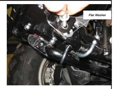
13. Install 6mm U-bolts, lock nuts, and flat washers around front tube and through fairlead mount bracket.
