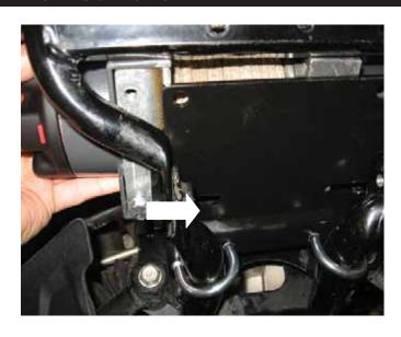
7. Slide winch toward center while aligning bolt and washer with slot. Slide until the end of the slot is reached. Install a second 8mm x 20mm long bolt and lock washer from Warn winch kit.
