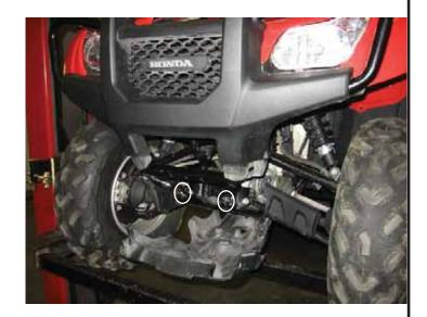
3. Remove front plastic guard and loosen four upper factory front tube bolts.
