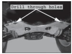
Figure 5 Drill through SkidPlate
