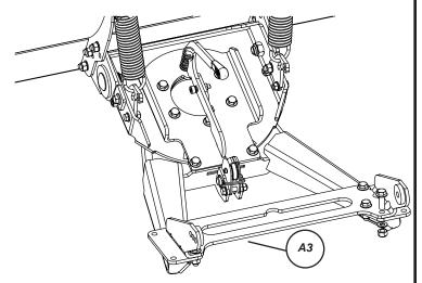
Figure 4 Install Plow Mount Flange
